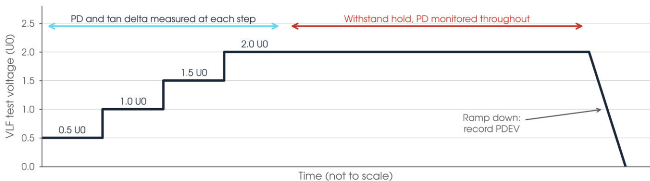
Illustrative sequence. Withstand level and hold time: IEEE 400.2-2024 cl 5.1.1 or the asset owner's specification.
